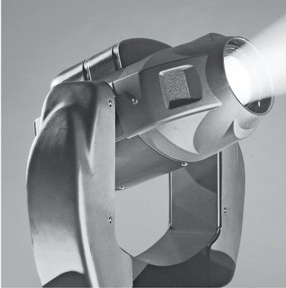
The VARI\*LITE® VL2202™ spot luminaire is based on the VL2201™ spot luminaire. The VL2202 luminaire features an upper enclosure that houses the control electronics as well as a power factor corrected arc power supply for the 700 watt short arc lamp. The VL2202 luminaire also features a zoom lens system and rotating gobos. The luminaire is small, fast, lightweight and virtually silent.
